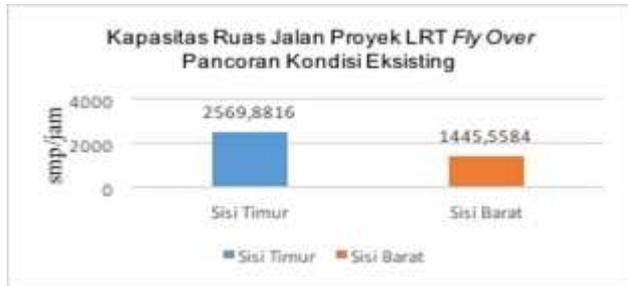
**Gambar 3.** Kapasitas Ruas Jalan Proyek LRT Fly Over Pancoran Kondisi Eksisting
