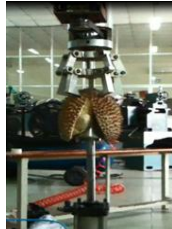
Figure 14. Durian husking separation testing
