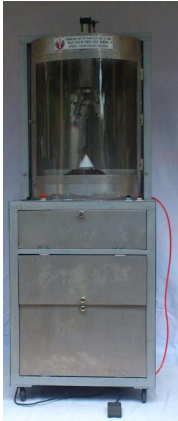
Figure 12. Manufactured semi-automatics durian defleshing machine
