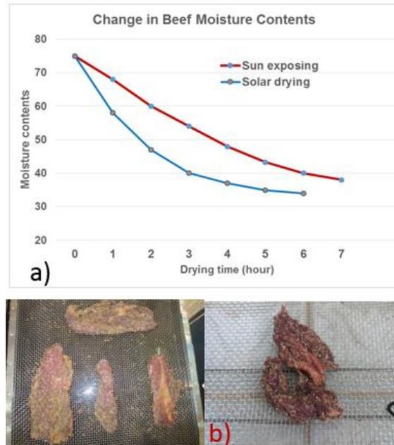
**Figure 10.** The change in MC (a) and colour of beef (b) dried by solar dryer
