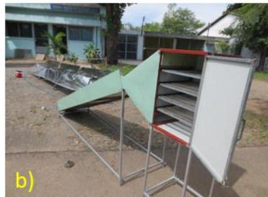
**Figure 5.** Solar dryer using for investigation, a) Schematic, and b) manufactured solar dryer.
