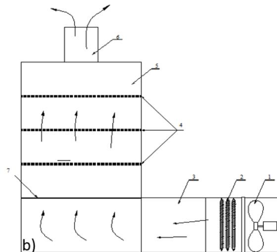
**Figure 3.** The hot air dryer a) completed manufactured dryer and b) components schematic.
