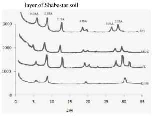
Figure9:X-ray diffractgram of clay fraction from surface layer of Tazeh kand soil
