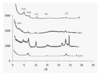
Figure 7:X-ray diffractgram of clay fraction from surface
