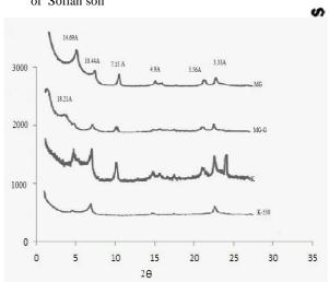
Figure 3:X-ray diffractgram of clay fraction from surface layer of Baranlo soil
