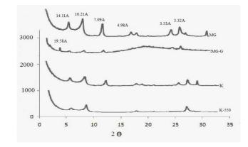
Figure 11:X-ray diffractgram of clay fraction from surface layer of kozeh kanan
