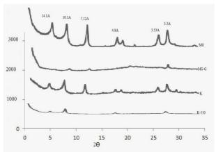
Figure 5:X-ray diffractgram of clay fraction from surface layer of Gharamolk soil
